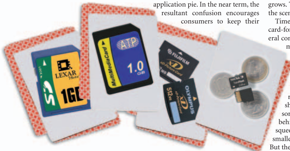
Figure 1 A multiplicity of memory cards awaits your evaluation; among them, from left to right, are SD Card, MultiMediaCard, xD-Picture Card, and TransFlash.
