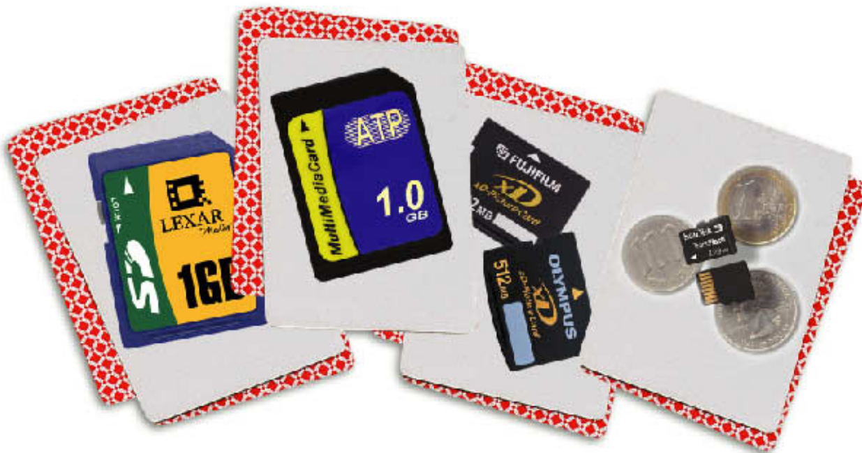
A multiplicity of memory cards awaits your evaluation; among them, from left to right, are SD Card, MultiMediaCard, xD-Picture Card, and TransFlash.
