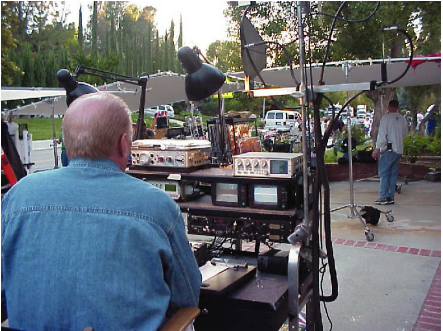
A sound mixer on the set of CSI: Miami connects stationary and wireless microphones to the Deva II audio-recording unit.
