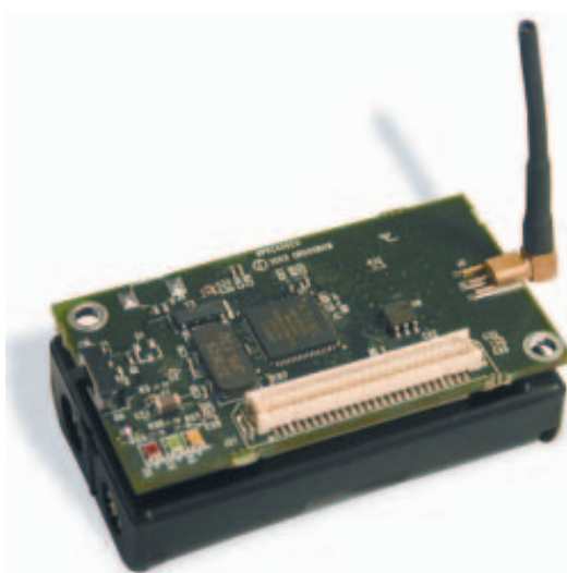
Figure 4 Crossbow Technology offers the MICAz RF transceiver, which bridges the gap between its extensive sensor-network products and the emerging ZigBee standard.
