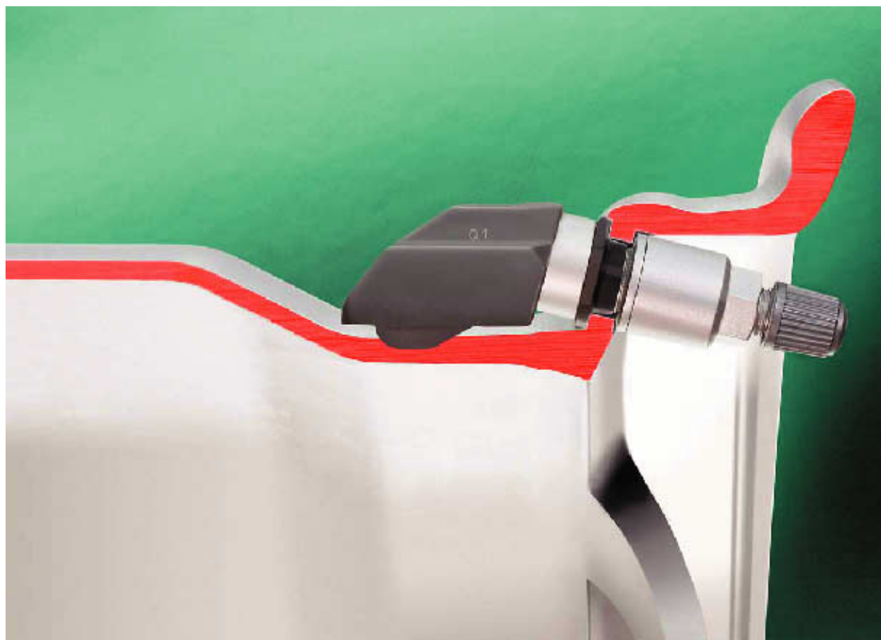
Beru's sensor module mounts inside the tyre on the valve stem.
