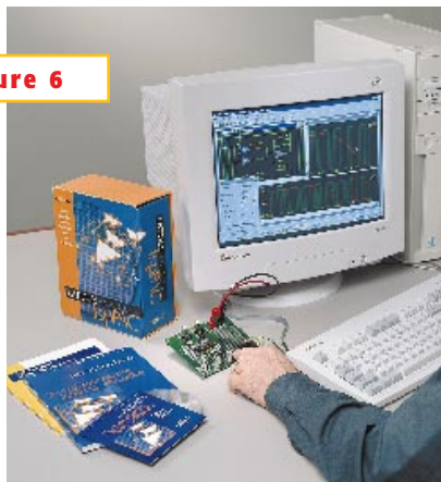
You program the ispPAC10 series with a design kit that includes PC-based software, two IC samples, and an evaluation board.
