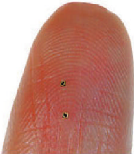
A fingertip dwarfs Hitachi's \mu -Chips, which are a fraction of the size of a grain of rice (courtesy Hitachi).
