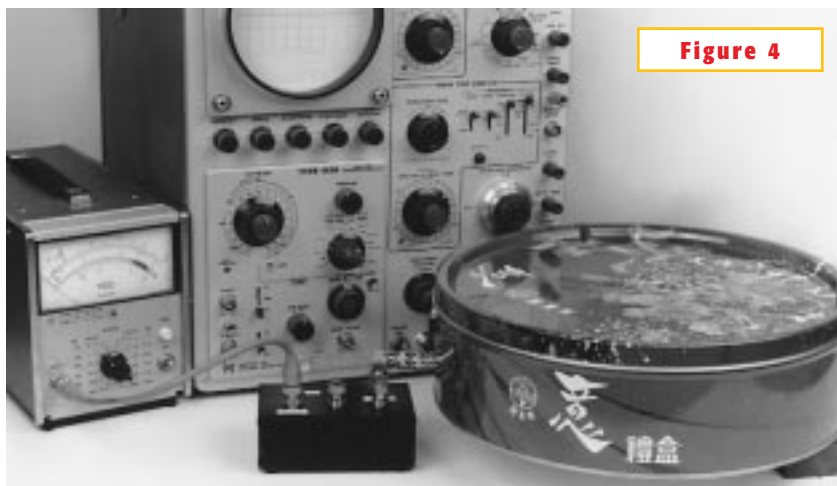
A shielded can contains the regulator, and the noise filter circuitry occupies the small black box. The oscilloscope and rms voltmeter never connect to the test set simultaneously, precluding a ground loop from corrupting the measurement.
