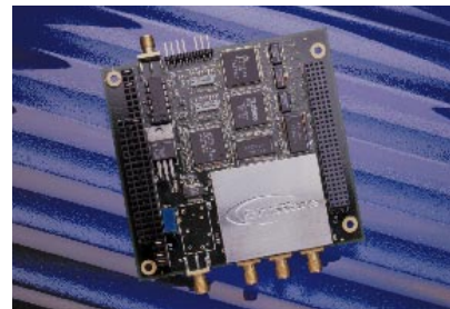
The $2995 DDR-bitsi digital drop receiver from BittWare Inc contains four independent down-conversion channels for high-accuracy software-radio applications.
