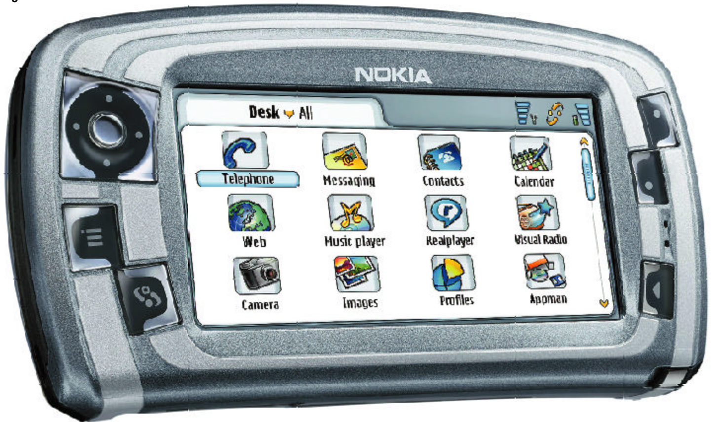
The Nokia 7710 smart phone runs the latest Symbian Series 90 operating system and features a landscape 640 × 320-pixel, color touchscreen display.
