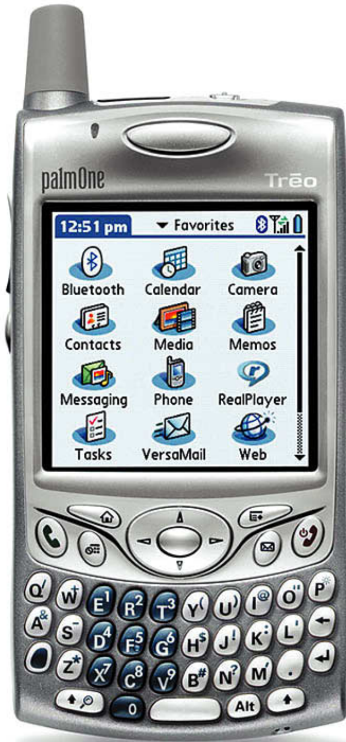
The Treo 650 from PalmOne combines all the features of the popular PDA plus Internet access, e-mail, and a GSM or CDMA cellular connection.
