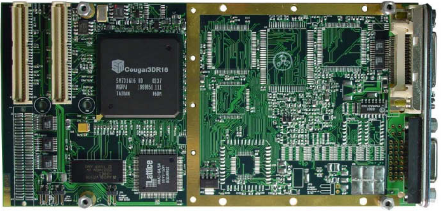
The new Topaz/PMC card combines VGA/LVDS/DVI graphics with video, DVI, and RGB digitizers.
