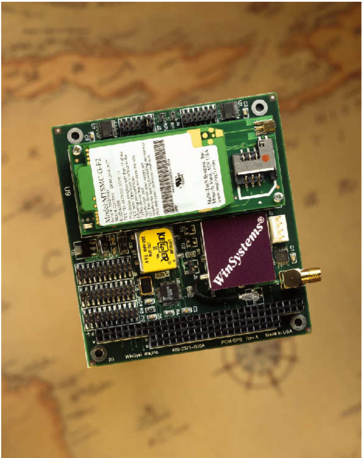
With both GPS and cell-modem support, the PCM-GPS delivers navigation and communication functions for mobile applications.
