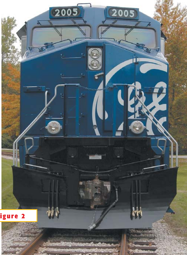
The clean lines and the sheer size of GE Transportation’s 4400-hp Evolution Series locomotive are impressive.
