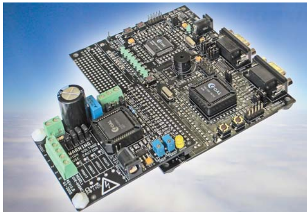
A new evaluation system for the HVDAC200-4 quad, high-voltage D/A converter features a local 8051 controller and PC-based demonstration and development software.
