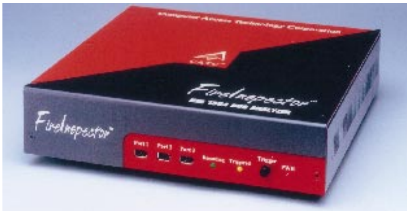
The FireInspector PC-based bus/protocol analyzer from CATC scrutinizes the IEEE 1394 high-speed serial bus.
