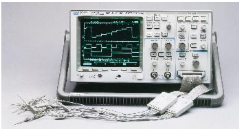
For hardware debugging, a scope is almost indispensable, but using a separate scope and logic analyzer can become messy. However, a few low-cost instruments combine the two functions. HP's $4995 54645D combines two 100-MHz scope channels with 16 logic-timing-analysis channels.
