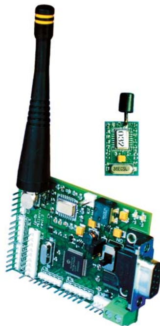
Smart-sensor wireless networks, such as Millennial Net’s 916-MHz product family, must operate in remote locations, where changing the battery is not an option. The power requirement for the small end node (upper right) is on the order of microamps.
