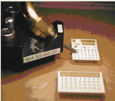
Figure C Instrument calibration at the probe tips uses a precise impedance-standard substrate.
