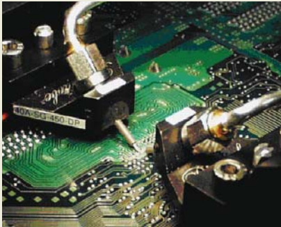
Figure A You can easily measure the properties of interconnects, such as differential traces on a pc board, without introducing impedance discontinuities, such as those that can occur with SMA connectors.
