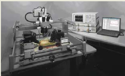
Figure B A flexible probing system allows accurate measurement of a wide variety of interconnect hardware.
