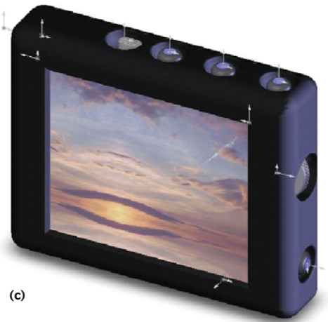
Figure 3 If imitation is the sincerest form of flattery, then Apple must be pleased with Luxpro's Super Tangent (a), whose looks are reminiscent of an iPod Shuffle (b). PortalPlayer's flash-memory-based reference design takes a different tack, with a color display and still-image capabilities (c).
