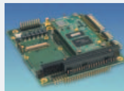
The OrbiTrak 8R provides GPS location data for vehicle-navigation, telematics, and fleet-management applications in a rugged, PC/104 form factor.
