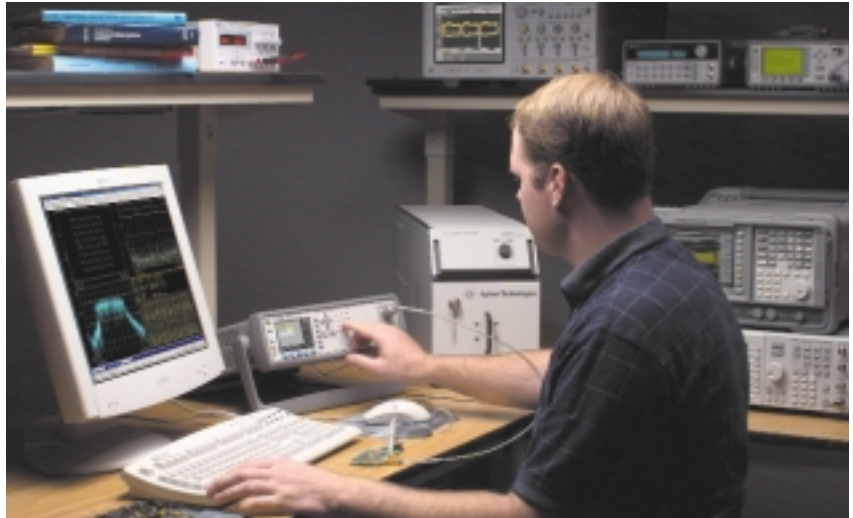
Testing a WiFi design requires a combination of RF- and data-level test equipment that designers must use together to fully exercise the protocols (courtesy Agilent Technologies).
