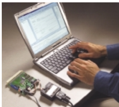
Silicon Labs' $199 development kit includes an Si8250-based half-bridge dc/dc target board; a real-time firmware kernel; and automated development tools.
