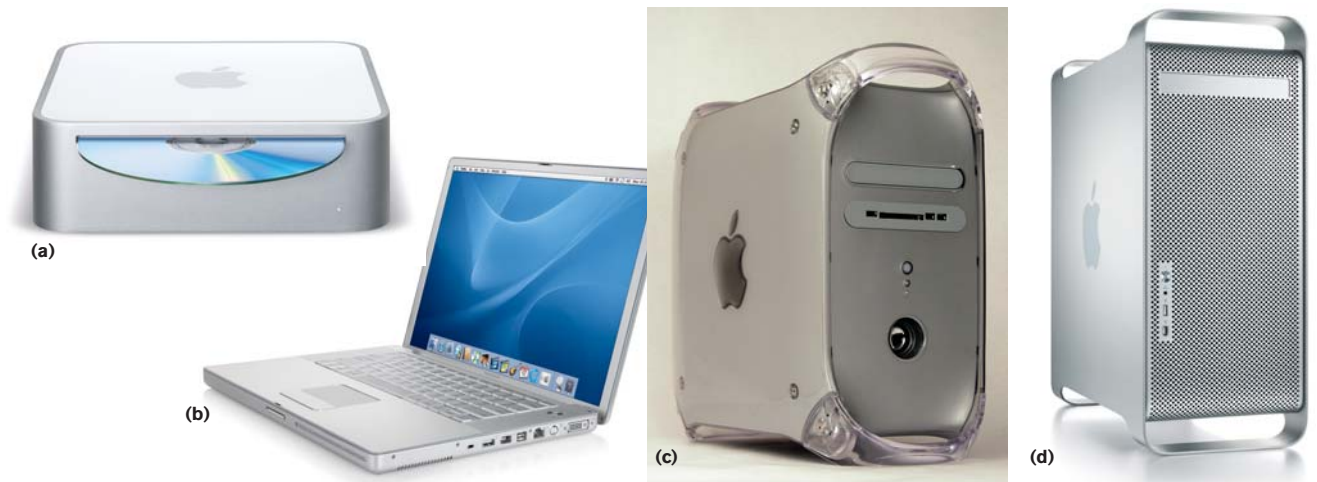
Figure 1 Apple's 1.25-MHz Mac Mini (a), 1.25-GHz G4 PowerBook (b), dual 800-MHz G4 Quicksilver Power Mac with GeeThree's Sweet Multiport installed (c), and dual 1.8-GHz G5 Power Mac (d) underwent intensive benchmark scrutiny during this hands-on project.
