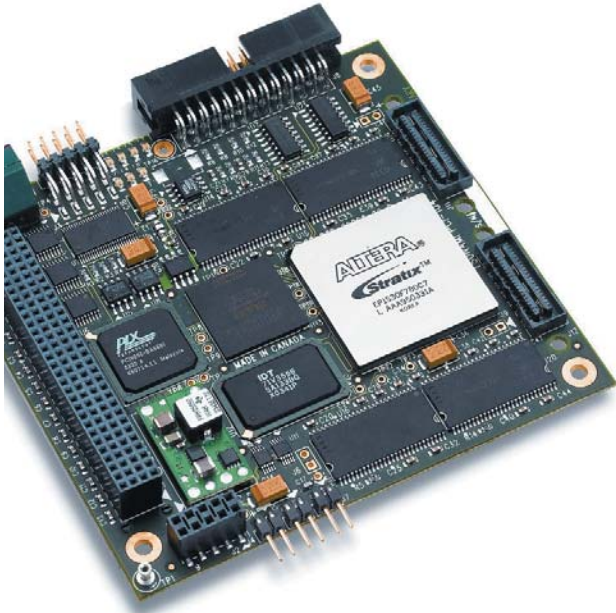
Figure 4 The Tsunami PC104 platform from SBS Technologies gives users an Altera Stratix FPGA on a 32-bit, 33-MHz PCI interface for custom processing.
