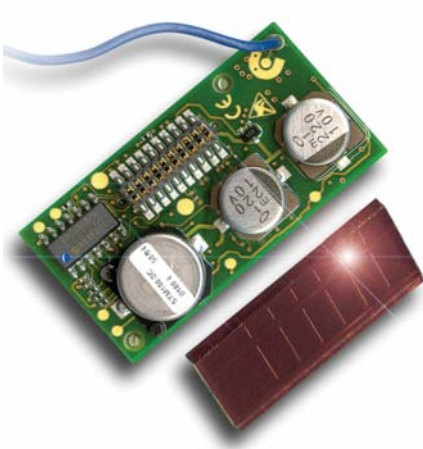
Figure 3 The solar cell that powers EnOcean's STM100 network-transmitter node has two sections: The square area on the left charges a conventional capacitor, and the larger area on the right charges an ultracapacitor.
