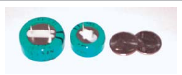
Figure 2 Supercapacitors from NEC America provide 1F (left) and 0.5F of storage at 5.5V maximum and occupy little pc-board area.
