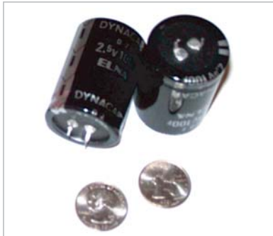
Figure 3 These 100F, 2.5V Dynacaps from Elna approximate standard electrolytic capacitors in volume.
