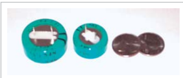
Figure 2 Supercapacitors from NEC America provide 1F (left) and 0.5F of storage at 5.5V maximum and occupy little pc-board area.
