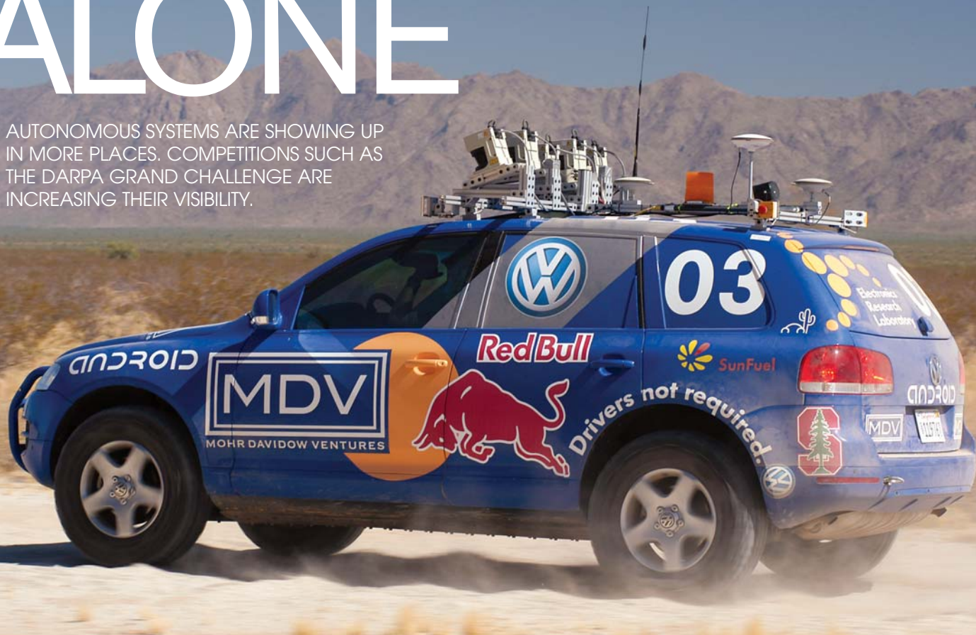
Figure 1 Stanford Racing Team's autonomous vehicle, “Stanley”—a reinforced Volkswagen Touareg with a custom drive-by-wire system, a sensor rack, and a computing system—won the 2005 DARPA Grand Challenge (courtesy Stanford Racing Team).
