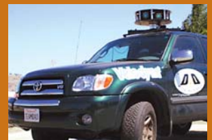
Figure A The custom LADAR system sits atop the vehicle driver cab and spins at 600 rpm to provide accurate terrain data (courtesy Team DAD).
