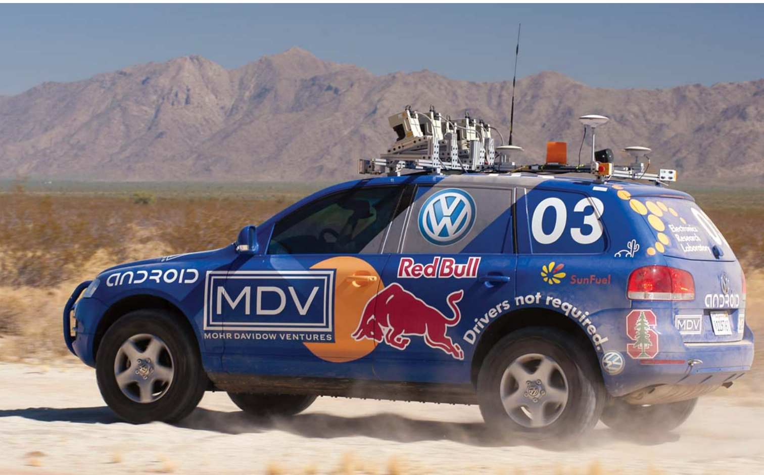
Figure 1 Stanford Racing Team's autonomous vehicle, "Stanley"—a reinforced Volkswagen Touareg with a custom drive-by-wire system, a sensor rack, and a computing system—won the 2005 DARPA Grand Challenge (courtesy Stanford Racing Team).
