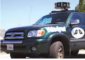
Figure A The custom LADAR system sits atop the vehicle driver cab and spins at 600 rpm to provide accurate terrain data (courtesy Team DAD).
