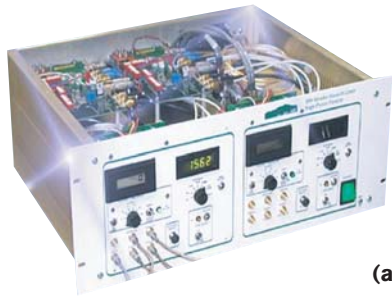
Figure 5 The custom-built, single-photon detector unit, which IBM Almaden built, has an optical-detector front end (a) and a considerable amount of support electronics (b).
