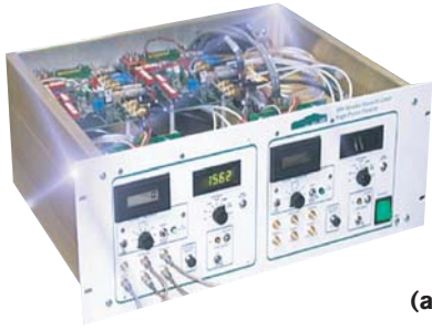
Figure 5 The custom-built, single-photon detector unit, which IBM Almaden built, has an optical-detector front end (a) and a considerable amount of support electronics (b).
