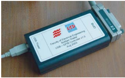
Figure 3 The controller in its housing presents a profile that's not much larger than a GPIB cable connector.
