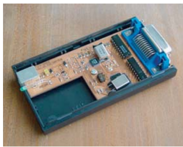
Figure 2 A top view of the controller's pc board shows the USB connector (left) and the GPIB connector (right).
