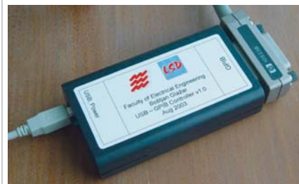
Figure 3 The controller in its housing presents a profile that's not much larger than a GPIB cable connector.
