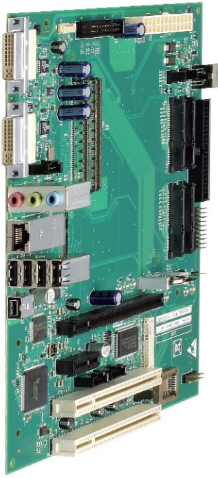
Figure 3 The Procelerant CR100 Flex ATX carrier board from Radisys serves as a COM Express development platform or carrier-board baseline.
