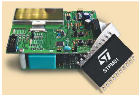
Figure 3 Combined with the STPM01 metering chip, a powerline modem provides a complete automatic power-meter solution.
