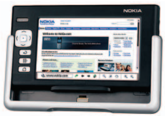
Figure 3 The $360 Nokia 770 Internet Tablet delivers wireless connectivity, an 800×480-pixel touchscreen, and 64 Mbytes of available flash memory.
