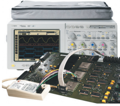
Figure 4 Agilent's FPGA probing option, together with Xilinx software, allows you to probe internal nodes of an FPGA as though it were a conventional logic PCB.
