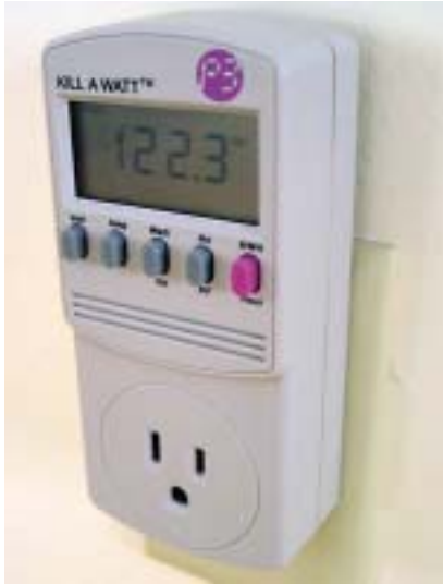
Figure 2 The low-cost Kill A Watt enables you to easily and accurately measure system power consumption in various operating modes.
