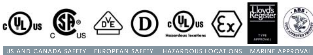
Figure 5 Product-certification marks are independent, third-party evidence of compliance and are mandatory in some localities.
