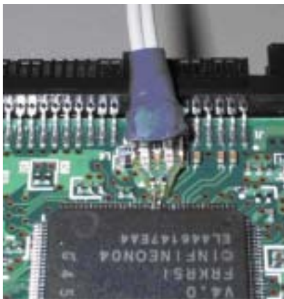
Figure 1 A differential active probe with 13-GHz bandwidth connects to the transmitter-package pins on a high-speed serial link.
