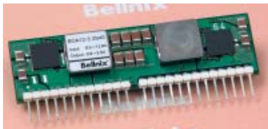
Figure 1 Designers usually dismiss point-of-load supplies as too simple to benefit from digital-control techniques, but this 40A supply from Bellnix incorporates a Volterra digital controller for less than $30.
