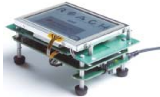
Figure 4 A new, 4-in., color, touch-display module from Reach Technology allows designers to integrate graphics as an intelligent serial device.
