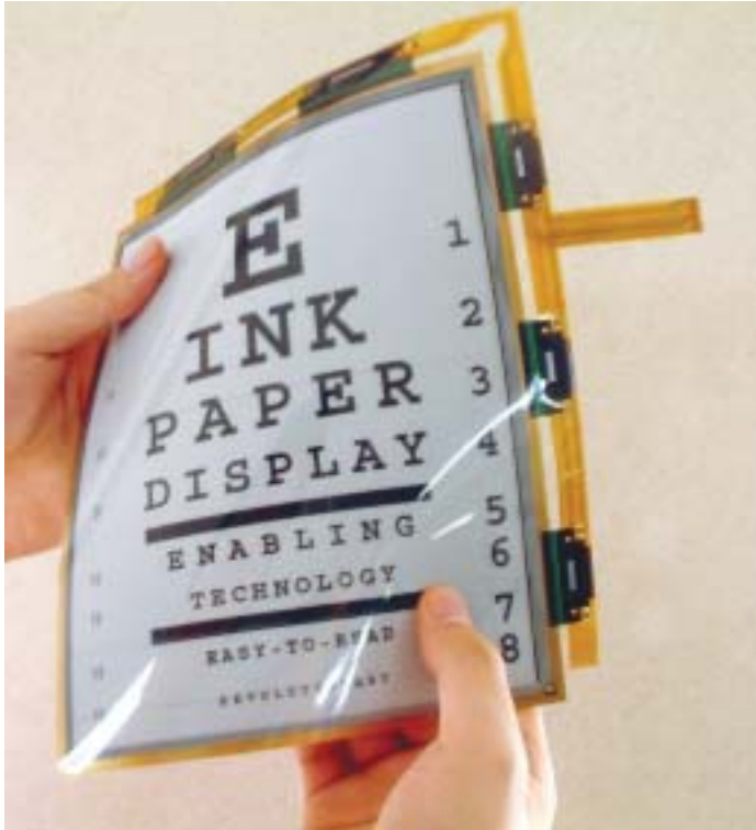
Figure 1 Electronic-paper displays from E Ink contain millions of bistable microcapsules that change color with an activating charge.
