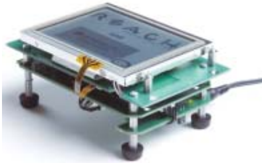
Figure 4 A new, 4-in., color, touch-display module from Reach Technology allows designers to integrate graphics as an intelligent serial device.
