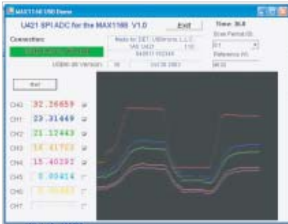
Figure 2 User-interface software for the data-acquisition system allows selection of operating parameters. In this image, the lower three channels are unselected and hence are not visible in the display.
