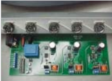
Figure 3 This version of the circuit comprises three constant-current driver channels. An LED light-bar assembly is above the pc board.
