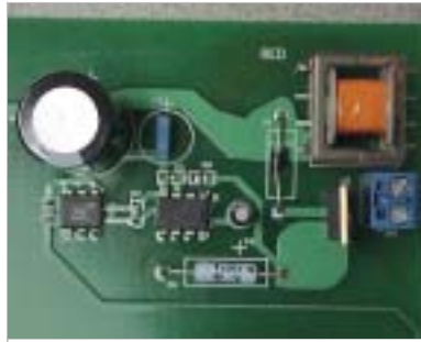
Figure 2 A close-up view of the circuit of Figure 1 shows inductor L_1 in the upper right corner.
