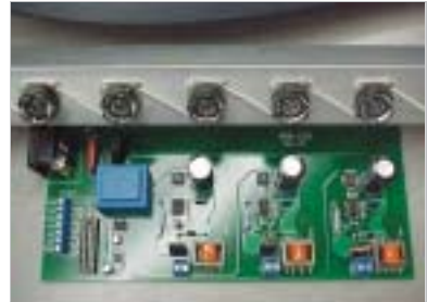
Figure 3 This version of the circuit comprises three constant-current driver channels. An LED light-bar assembly is above the pc board.
