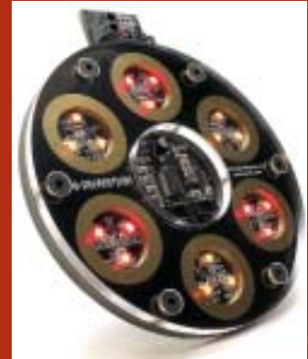
Figure C Quantum's QT160 six-key sensor offers stand-alone operation.
